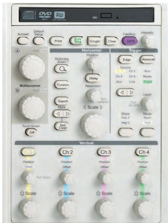
Figure 20. Front-panel control section of an oscilloscope.
