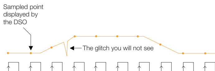
Figure 23. Sample rate varies with time base settings - the slower the time based setting, the slower the sample rate. Some digital oscilloscopes provide peak detect mode to capture fast transients at slow sweep speeds.
