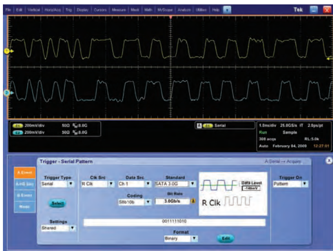
Figure 49. A DPO provides an ideal solution for non-repetitive, high-speed, multi-channel digital design applications.
