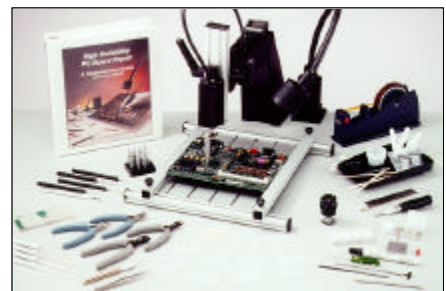
Figure 6: Bond the new edge contact with a Bonding System.
