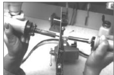
Figure 2: Place a soldering iron tip against the component lead and the desoldering tip over the lead end.
