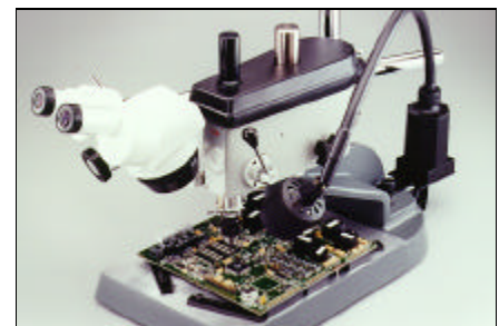
Figure 1: Precision Drill System with base plate to pin PC board in position while cutting inner layers.
