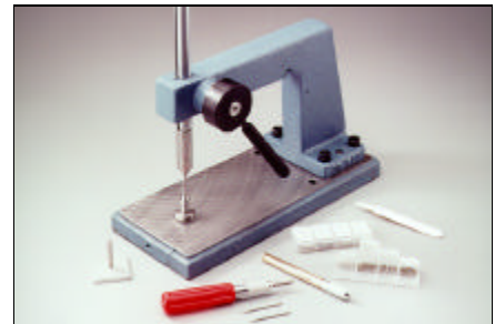
Figure 5: Set the eyelet using an Eyelet Press System.
